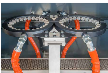
UVTREAT special pre treatment with pyrosil applied by double half ring burner.
