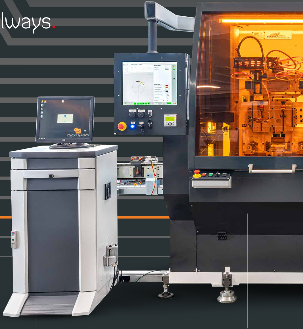
Matrix or linear camera for angular positioning or quality control
